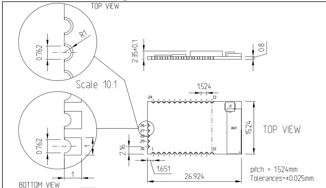
**Note:** An antenna area of 217X520 mils need to be free of any ground metallization or traces under the unit. The area extending away from the antenna should be free from metal on the PCB and housing to meet expected performance. Pin 25 is the required paddle ground and is not shown in this diagram.
