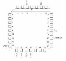
♦ You can connect this Combo-Debug-Card to any LPC bus. Some LPC interface chips are listed as below. You can connect the Combo-Debug-Card to the corresponding pins. For more information, please refer those chips' datasheets.
