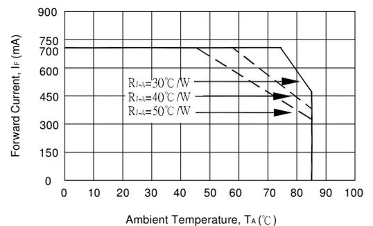
Note: Don't drive at rated current more than 5s without heat sink for Xeon 1 emitter series.
