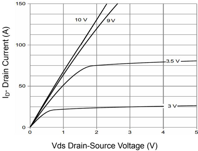
Figure 1 Output Characteristics
