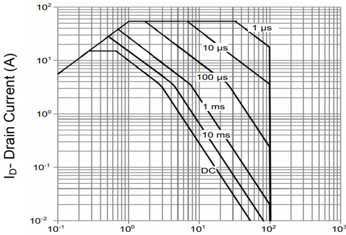
V<sub>ds</sub> Drain-Source Voltage (V)
