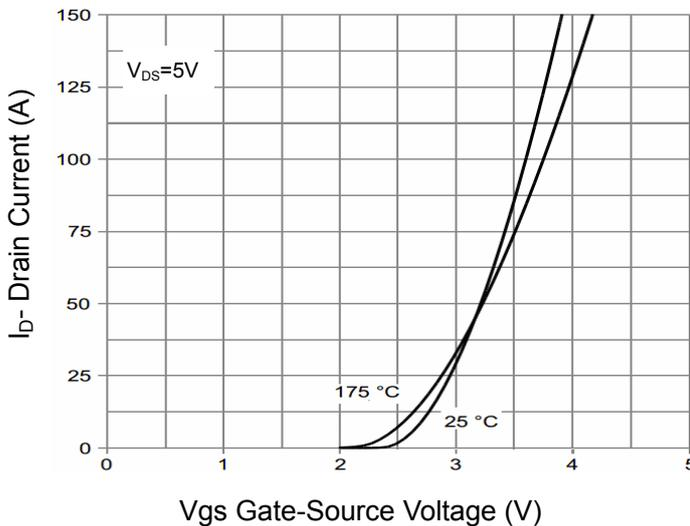
Figure 2 Transfer Characteristics
