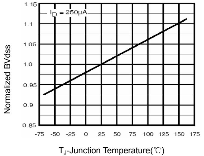
Figure 10 BV<sub>DSS</sub> vs Junction Temperature
