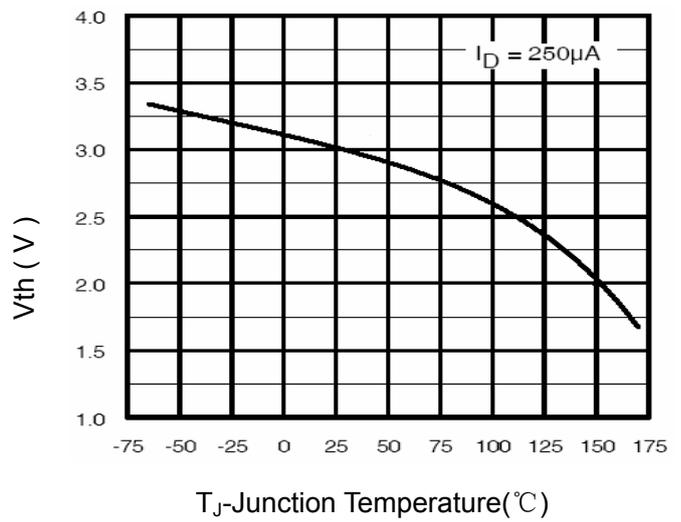
Figure 11 V<sub>GS(th)</sub> vs Junction Temperature
