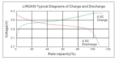
Charge: CC/CV 4.2V, 50mA(0.5C) Total 5hours Discharge: 50mA(0.5C) Cut-off at 3.0V Temperature: 25°C
