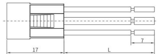
Connector: Cable length:150mm Other lengths can be customized
