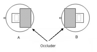
The sensitivity balance of dual element sensor is calculated through testing the sensitivity (single signal output voltage) of each element and using the following formula:
