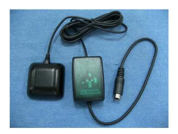
EverMore GM-R306-AA series is a high sensitivity GPS receiver, This product is based on EverMore chipset in 12 channel GPS receivers solution. The GPS module receiver will track up to 12 satellites at a time while providing fast time-to-first-fix and 1Hz navigation updates. It is far reaching capability meets the sensitivity & accuracy requirements of car navigation as well as other location-based applications, such as AVL system. PDA, Notebook operated navigation system.
