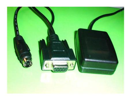
The GM-R305 GPS receiver provides EverMore's latest 12-channel GPS technology, contained inside a mouse-like box with a host connection cable.
